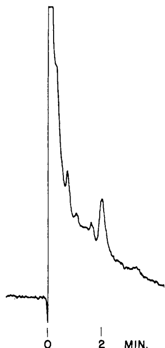
Figure 4. Gas chromatogram resulting from the analysis of the extract (obtained by following assay procedure) from a 3-day-off-drug liver (0.2 ppm). Column conditions same as for Figure 2
